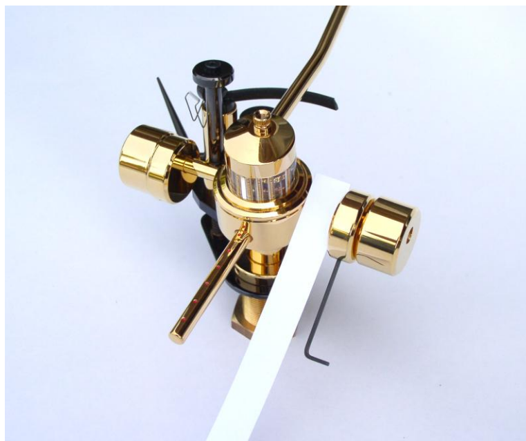
Fig. 5. Tightening the screw of the smaller weight on the other side.
