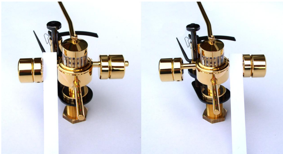
Fig. 7. The paper fits the spacing of the smaller weight adjusted at the VTA device and is used as spacing for the smaller weight on the other side.
