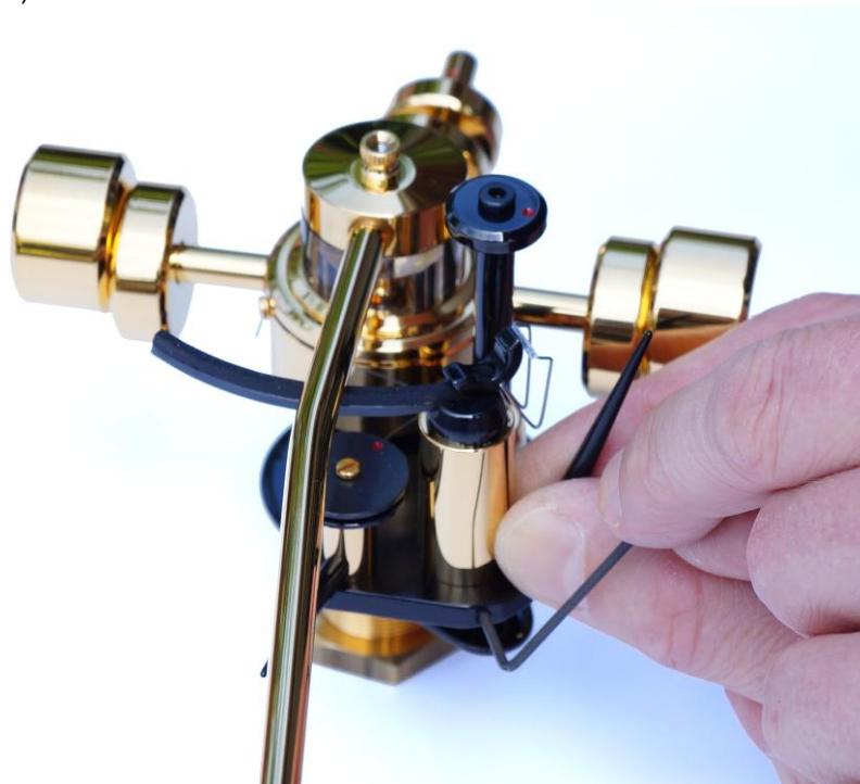
Fig. 11. Adjusting the height of the pickup lifter.
